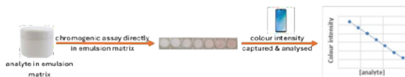
Fig. 1. Setup for the proposed extraction-free quantification methodology
